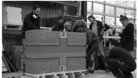
Bild 4: Mockup Atelier Boltshuser EPFL – Hybrid Beton-Lehm
